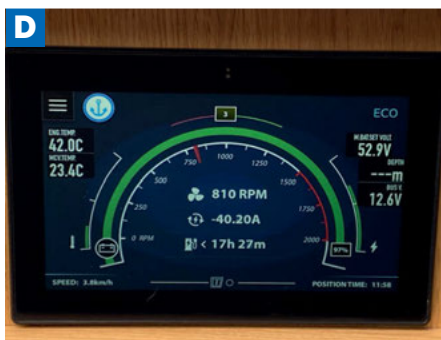
A A cover in the engine bay protects the electric motor frame and shorepower cable, as yet unused and still coiled. B The 200Ah 24V batteries being sized up before being fitted underneath the dinettes. C The electrics cupboard has a mass of well-ordered cabling and components in a ventilated space. D At cruising speed the motor is running around 800rpm, drawing 40A (around 2kW). E The 6.5kVA low-speed diesel generator is quiet and can quickly recharge the battery bank, if required, as well as heat the hot water.
