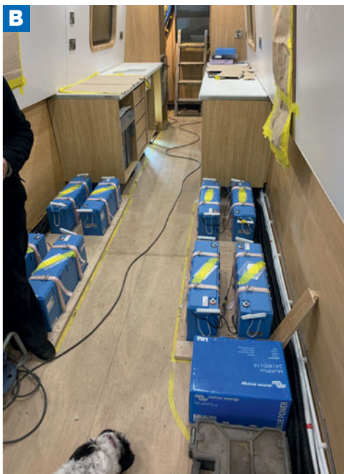
A A cover in the engine bay protects the electric motor frame and shorepower cable, as yet unused and still coiled. B The 200Ah 24V batteries being sized up before being fitted underneath the dinettes. C The electrics cupboard has a mass of well-ordered cabling and components in a ventilated space. D At cruising speed the motor is running around 800rpm, drawing 40A (around 2kW). E The 6.5kVA low-speed diesel generator is quiet and can quickly recharge the battery bank, if required, as well as heat the hot water.
